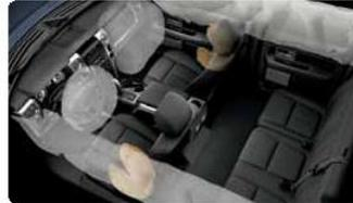
**THE NEW STANDARD SAFETY CANOPY SYSTEM** fully offers protection in certain side-impact collisions or rollover events. Its advanced side-curtain airbags with roll-fold technology can slide the side-curtain between the window glass and an occupant's head if they are leaning toward the glass. Newly designed front-seat side "H" bags (in yellow) help dissipate crash forces to help enhance protection of the chest in certain side-impact events.
