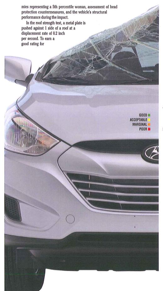
rollover protection, the roof must withstand a force of 4 times the vehicle's weight before reaching 5 inches of crush. This is called a strength-to-weight ratio.
